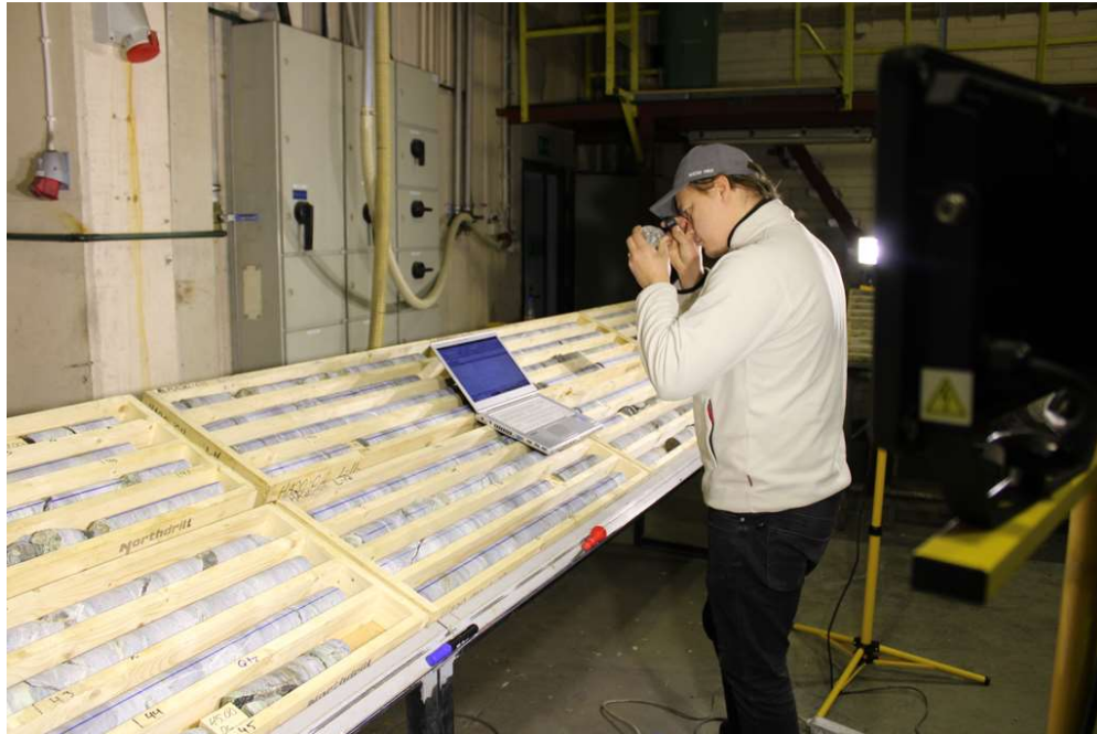
Figure 8-3 Geologist Kalle Penttilä logging drill core at FinnCobalts logging facility and warehouse in Outokumpu.
